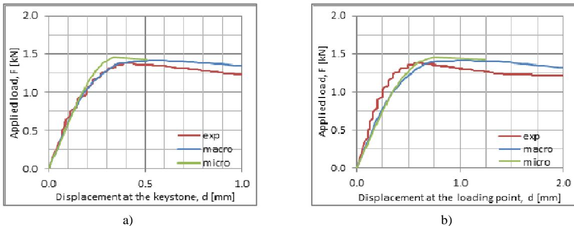
Figure 4: Comparison between experimental and numerical results presented on load - displacement curve at a) keystone, b) loading point.
