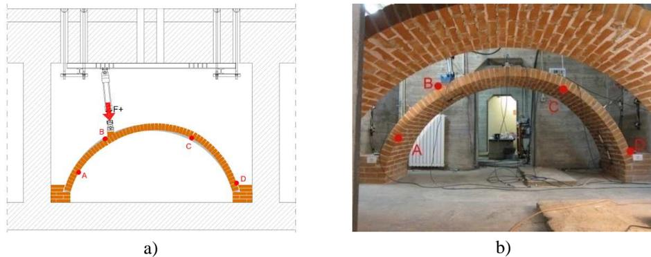
Figure 1: Unreinforced vault: a) scheme of the arch with location of plastic hinges; b) view of the location of plastic hinges[1].
