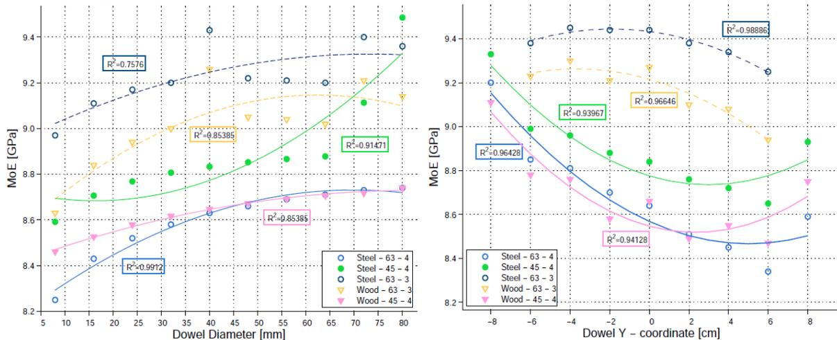
Figure 3: Results from the FE analyses; MOE depending on dowel diameter (left) and MOE depending on vertical position of dowel (right)
