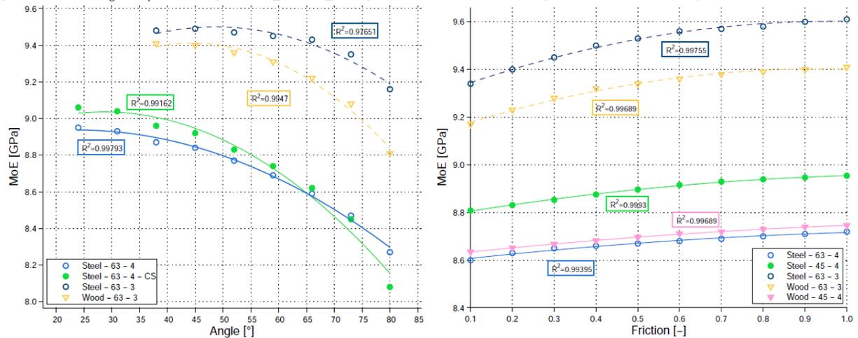
Figure 4: Results from the FE analyses; MOE depending on oblique face angle (left) and MOE depending on friction coefficient (right)
