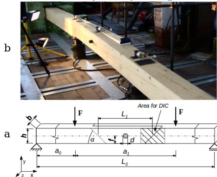
Figure 1: a) Geometry of tested beam and joint with oblique faces in 4-point bending test; b) tested sample of full-scale (testing was carried out with specimens oriented upside down)
