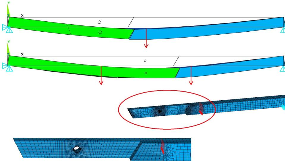
Figure 2: FE model of three-point bending and four-point bending; detail of the FE mesh
