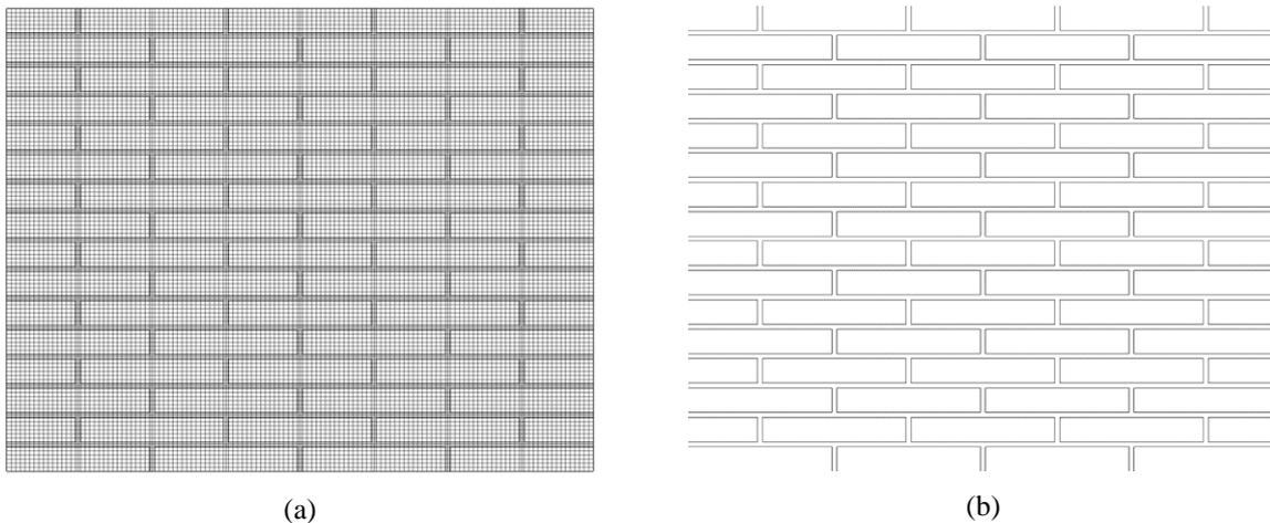
Figure 2: Finite element mesh: (a) continuum and (b) interface elements.
