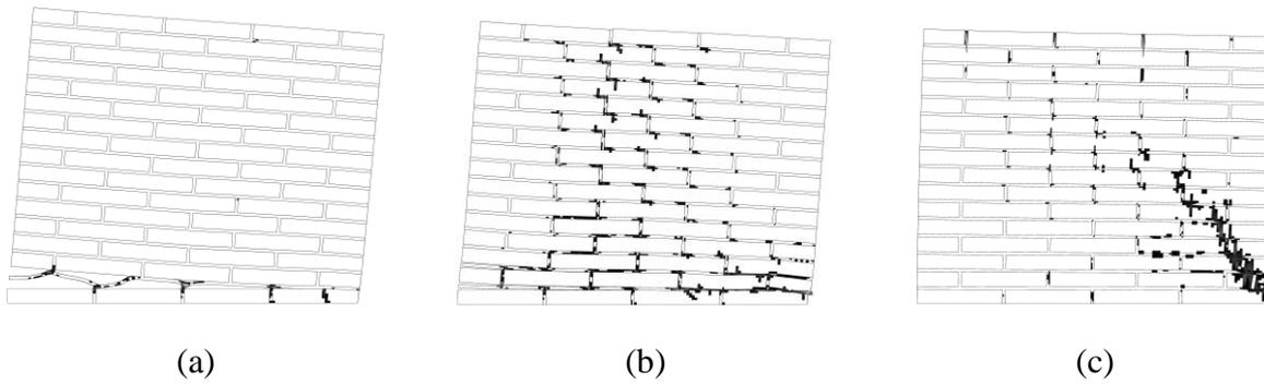
Figure 5: Failure mode examples. Deformation and tensile damage patterns for varying levels of vertical pre-stress: (a)  $\sigma = 0.893$  MPa, (b)  $\sigma = 2.981$  MPa and (c)  $\sigma = 9.048$  MPa.
