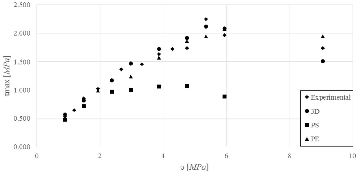
Figure 3: Interaction diagram comparison between experimental, 3D, plane stress and plane strain values.
