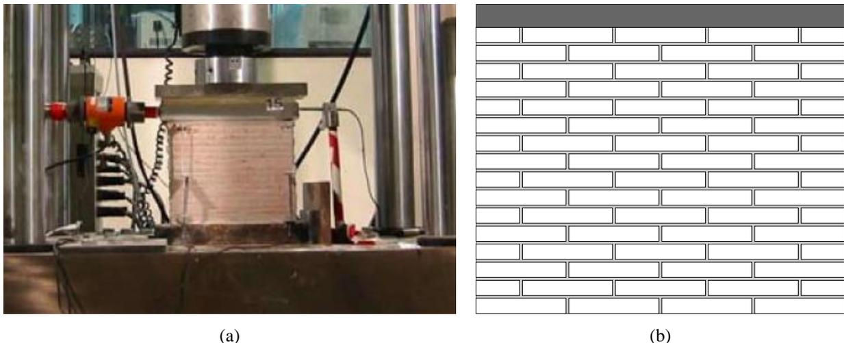
Figure 1: (a) Experimental setup and (b) wall geometry.
