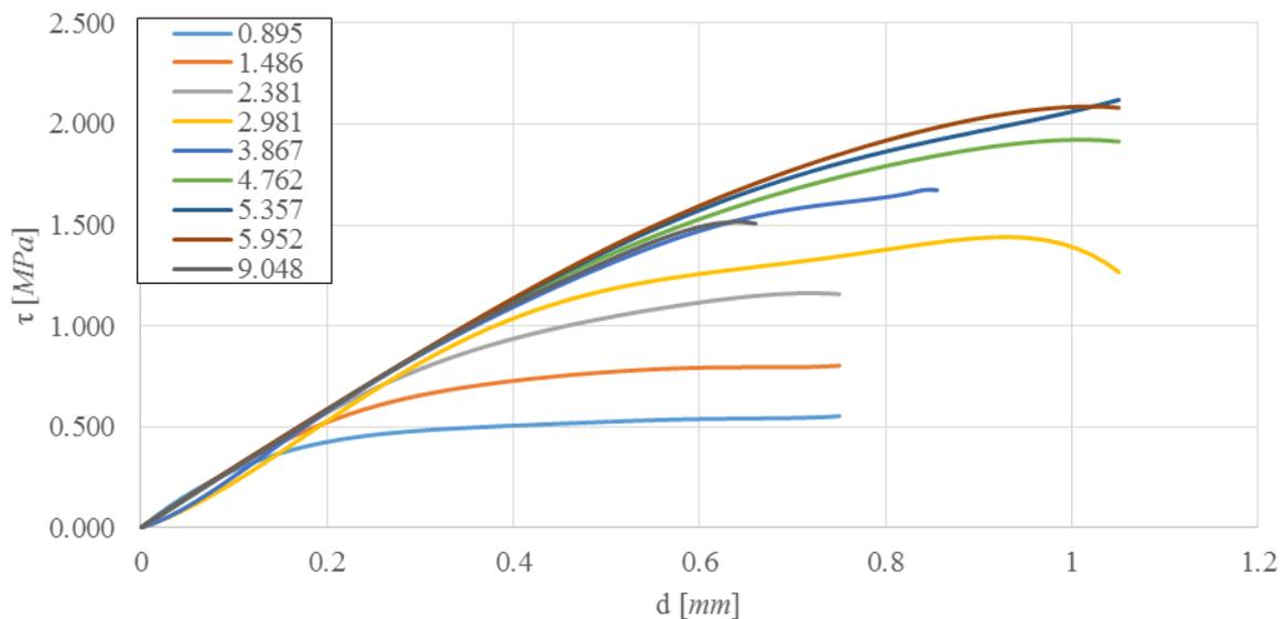
Figure 4: Shear stress-displacement diagrams for 3D model for various levels of vertical pre-stress.
