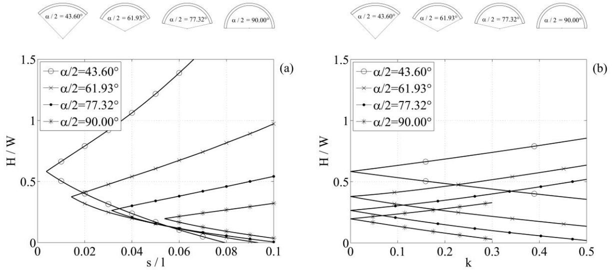
Figure 6: Normalized horizontal thrust for circular arches as function of the open angle  $\alpha$  and of dimensionless thickness  $s/l$  (a), the angle  $\alpha$  and of load multiplier  $k$  (b) (lower branch = left abutment thrust, upper branch = right abutment thrust).
