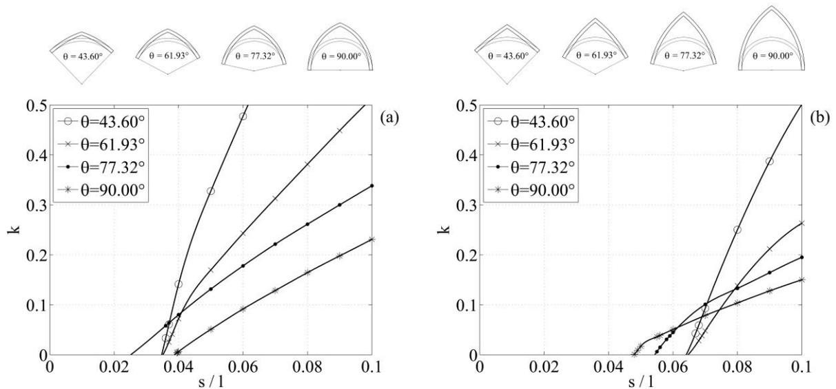
Figure 7: Load multipliers for pointed arches  $f/f_0 = 1.5$  (a),  $f/f_0 = 2$  (b).
