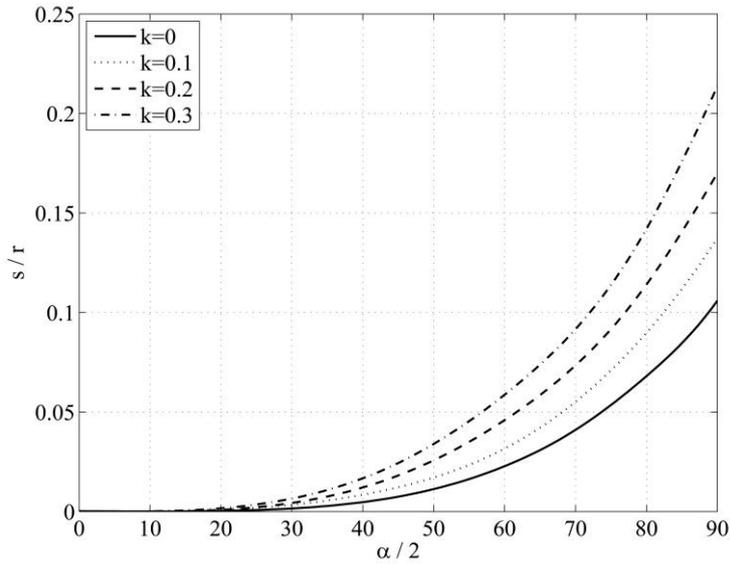
Figure 5: Minimum thickness for circular masonry arches with vertical and horizontal loads.
