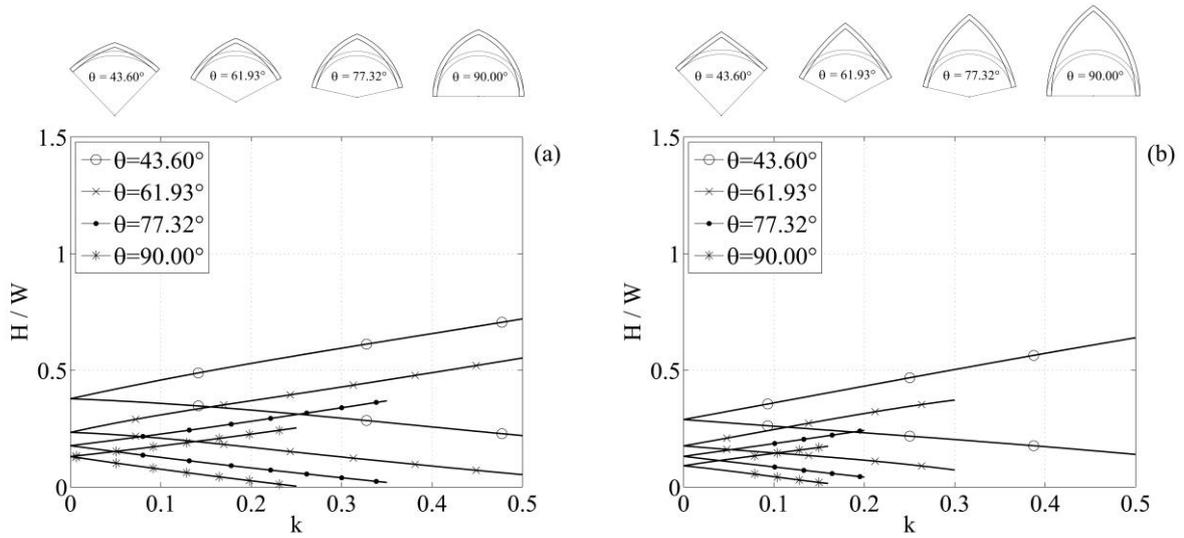
Figure 10: Normalized horizontal thrust for pointed arches  $f/f_0 = 1.5$  (a),  $f/f_0 = 2$  (b).
