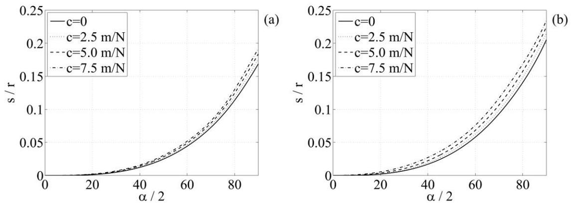
Figure 13: Minimum thickness for circular masonry arches with vertical and horizontal loads, at several values of flexibility - case  $k=0.2$  (a), case  $k=0.3$  (b).
