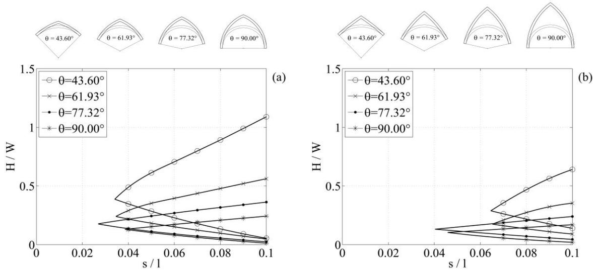
Figure 9: Normalized horizontal thrust for pointed arches  $f/f_0 = 1.5$  (a),  $f/f_0 = 2$  (b).
