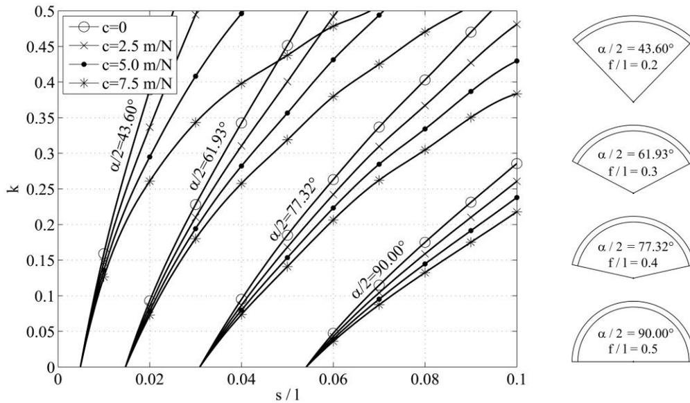
Figure 12: Load multipliers for circular arches as function of geometry and flexibility of abutments.
