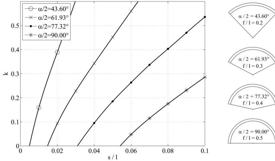
Figure 4: Load multiplier  $k$  of circular arches as function of geometry.
