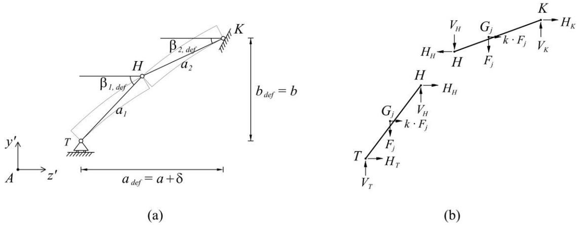
Figure 11: Kinematic description in large displacements (a) and forces acting on the two rigid links (b) - three hinged arch.
