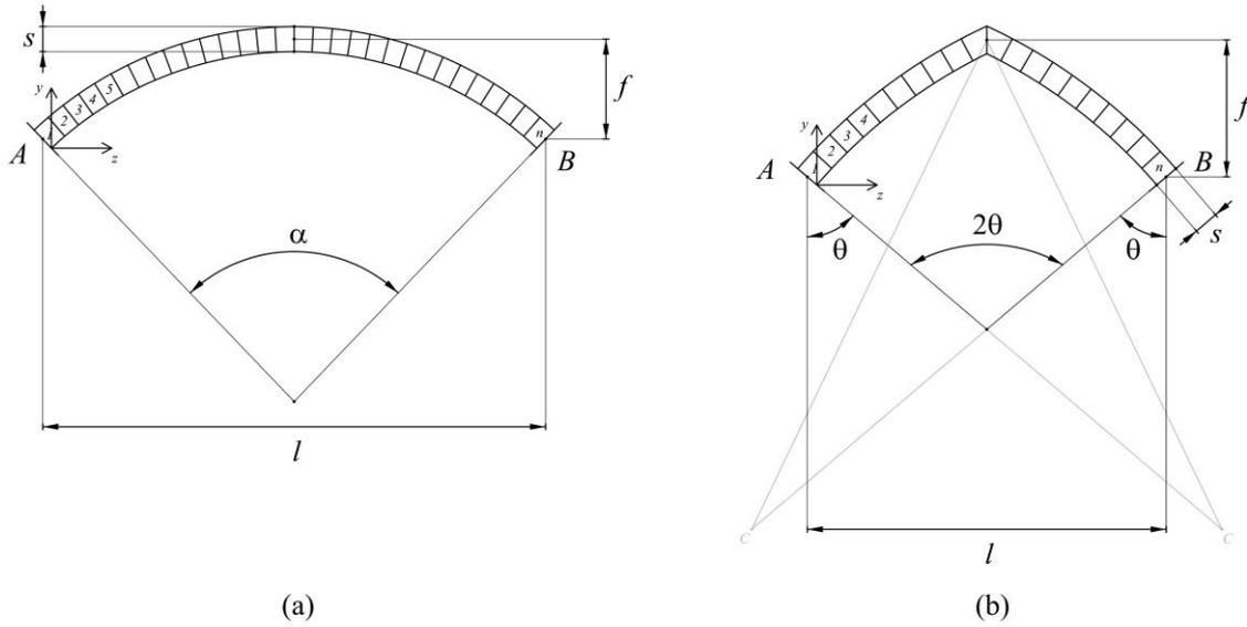
Figure 1: Geometry of circular (a) and pointed (b) masonry arch.
