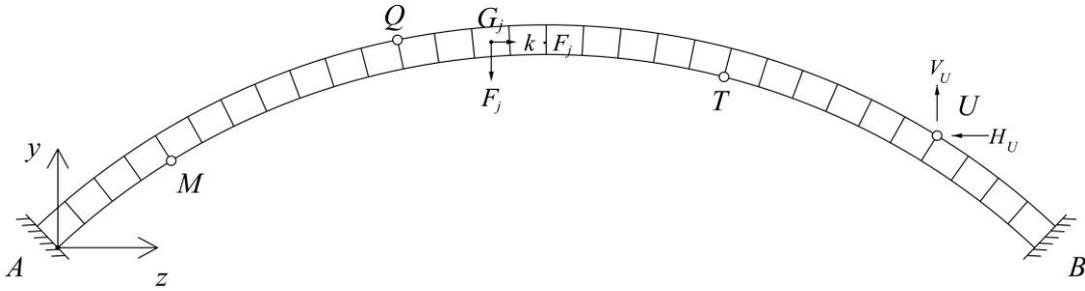
Figure 2: Generic four-hinge position associated to the collapse condition in the presence of vertical and horizontal loads.
