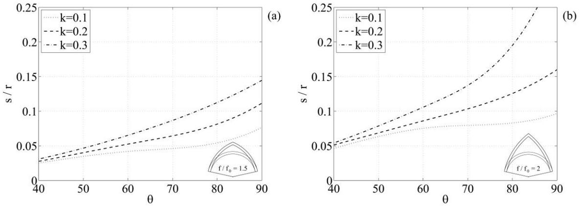
Figure 8: Minimum thickness for pointed masonry arches  $f/f_0 = 1.5$  (a),  $f/f_0 = 2$  (b).
