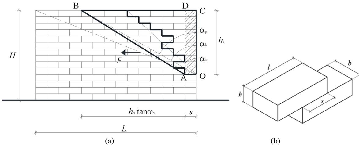
Figure 2: (a) Sidewall with inclinations for the unit ( $\alpha_b$ ) and wall shape ( $\alpha_p$ ) ratios and for the variable angle of crack ( $\alpha_c$ ). (b) Unit dimensions.
