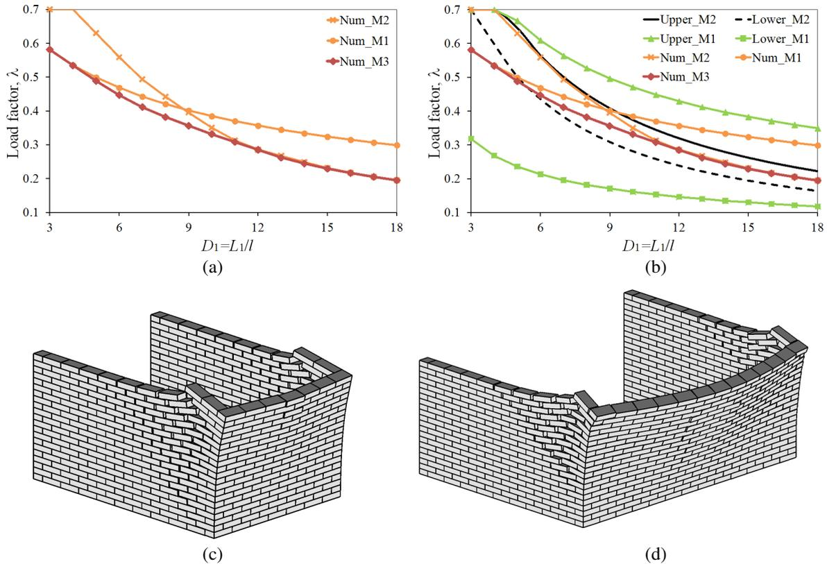
Figure 4: Size ratio effect. Load factors vs. size ratio of the front wall for (a) micro-block model, (b) micro and macro-block models. Micro-block failure mechanisms for M3, with (c)  $D_1 = 7$  and (d)  $D_1 = 13$ .
