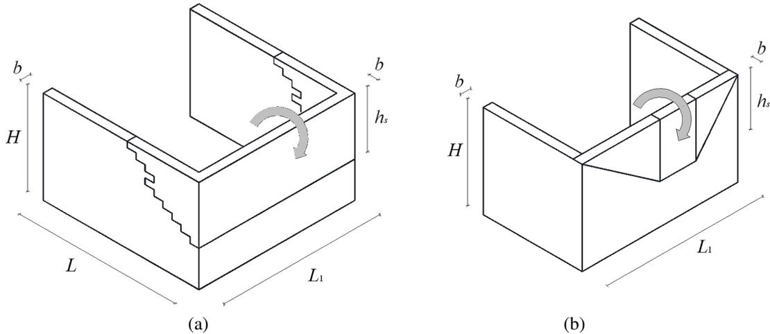
Figure 1: (a) Mechanism 1 with sliding-rocking failure of the sidewalls; (b) Mechanism 2 with twisting-sliding-rocking failure of the front wall.
