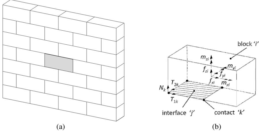
Figure 3: (a) Micro-block model; (b) static variables at block centroid  $i$ , and contact point  $k$ .
