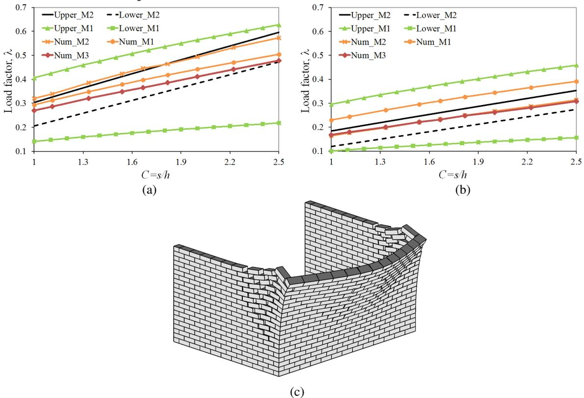
Figure 5: Unit aspect ratio effect. Load factors vs. unit aspect ratio for (a)  $D_1 = 7$  and (b)  $D_1 = 13$ . (c) Micro-block failure mechanisms for M3, with  $D_1 = 13$  and  $C = 1.5$ .
