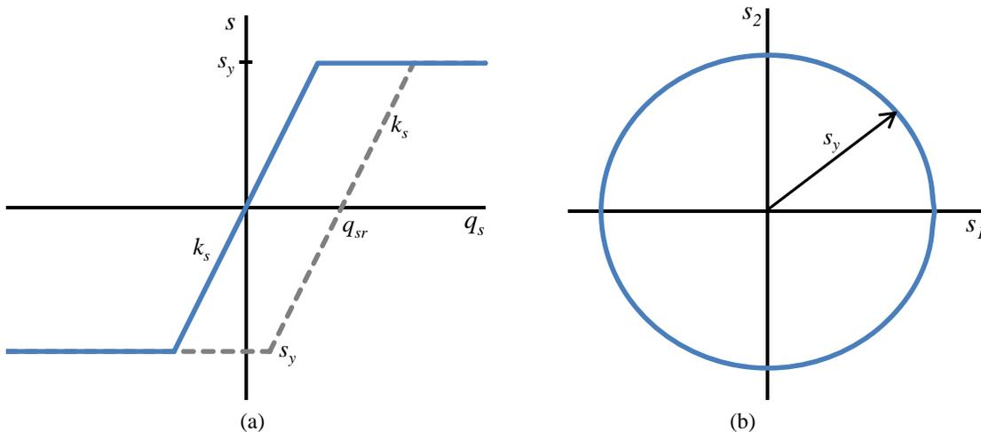
Figure 2: Shear constitutive model; (a) shear force vs. Sliding displacement curve and; (b) yield surface
