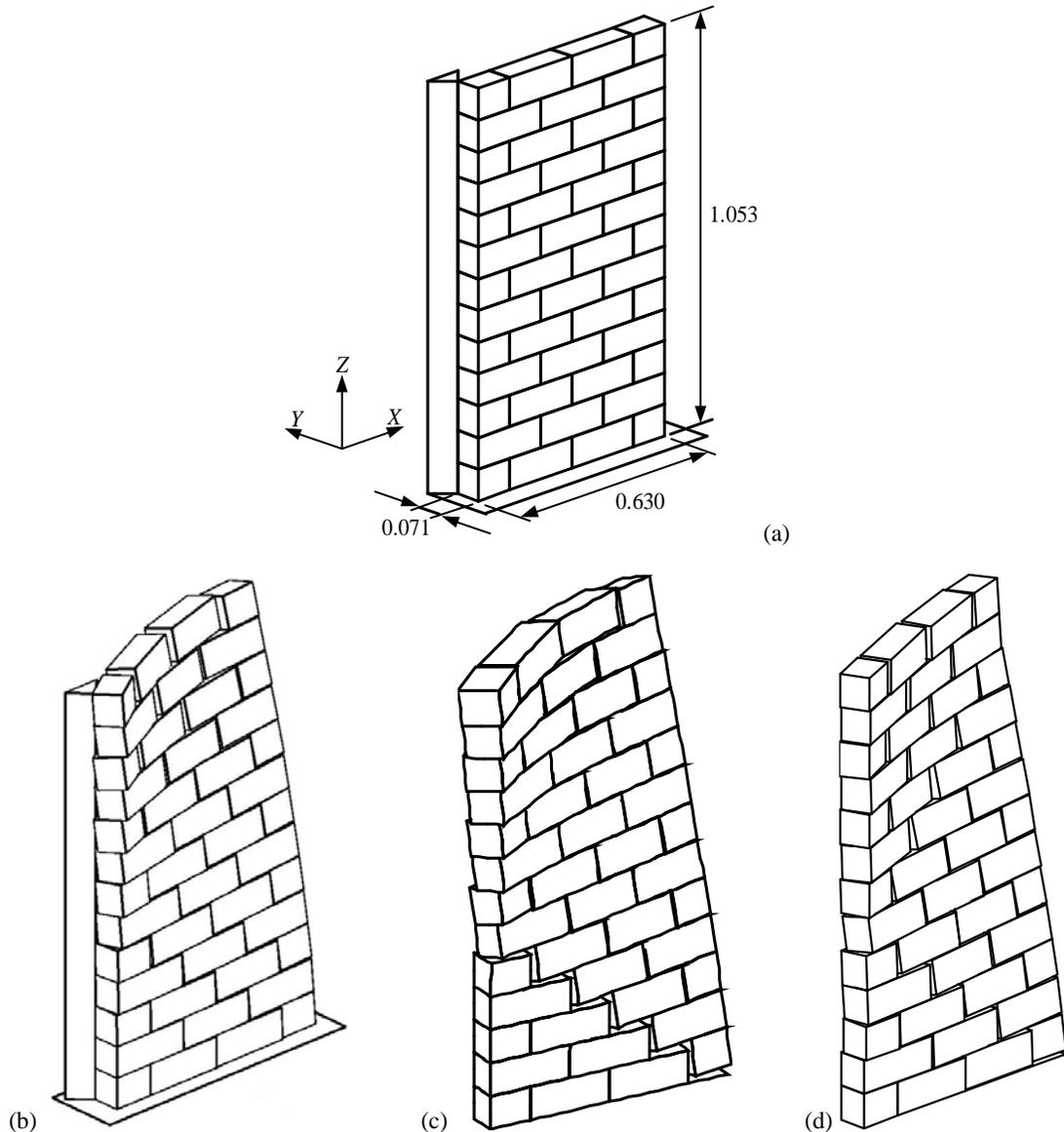
Figure 3: Dry-jointed masonry wall; (a) model; failure mechanisms by: (b) rigid block non-linear analysis; (c) FEM; (d) limit analysis
