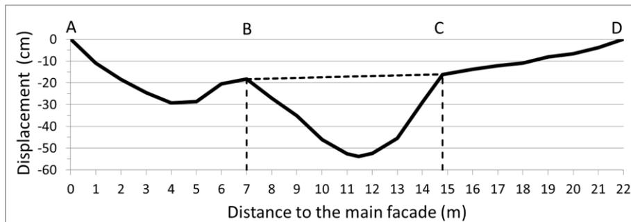
Figure 9: Sectional view of the main nave showing the deformation of arch and the loss of verticality of the walls.
