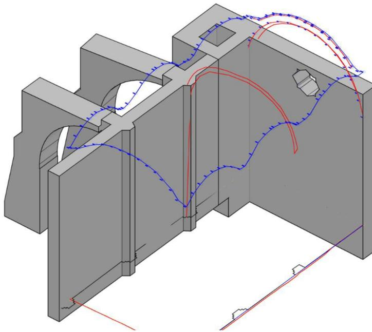
Figure 12: Geometrical model of the walls, tower and buttresses.
