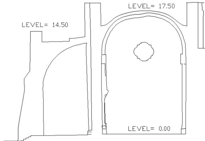
Figure 7: Sectional view of the main nave showing the deformation of arch and the loss of verticality of the walls.
