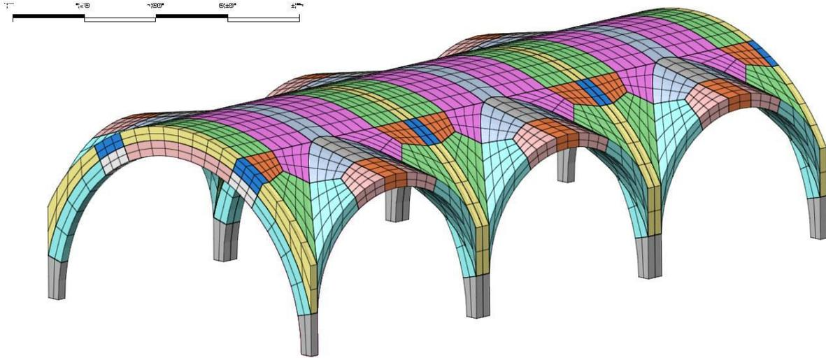
Figure 11: Structured mesh that models the vault and the arches with hexahedral elements.
