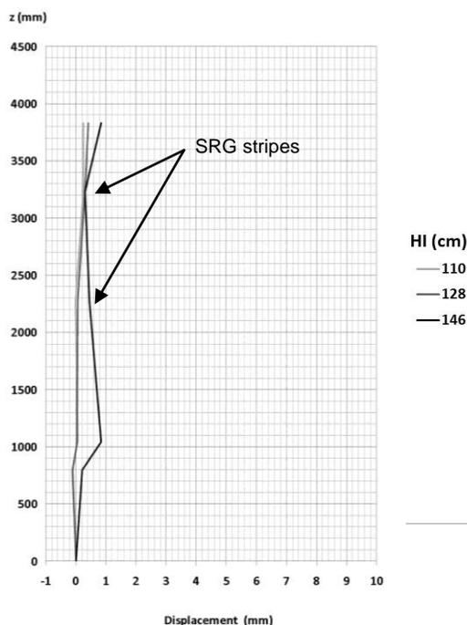
Figure 11: Evolution of south wall-façade connection in the three tests before collapse of the SRG reinforced specimen: displacements are limited in correspondence of the two SRG stripes.
