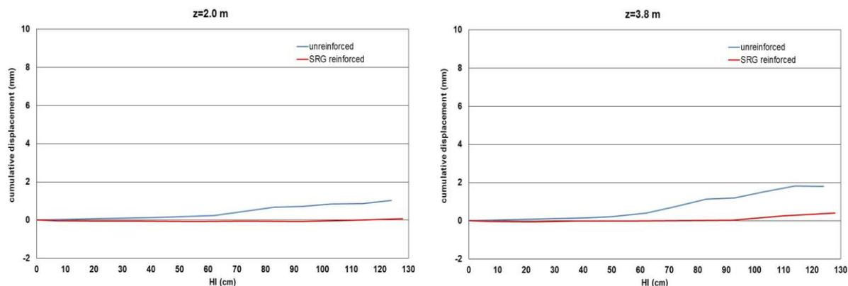
Figure 10: Evolution of south wall-façade connection at middle height (left) and on top (right) in function of the input HI along the test sequence on the unreinforced and SRG-reinforced specimen.
