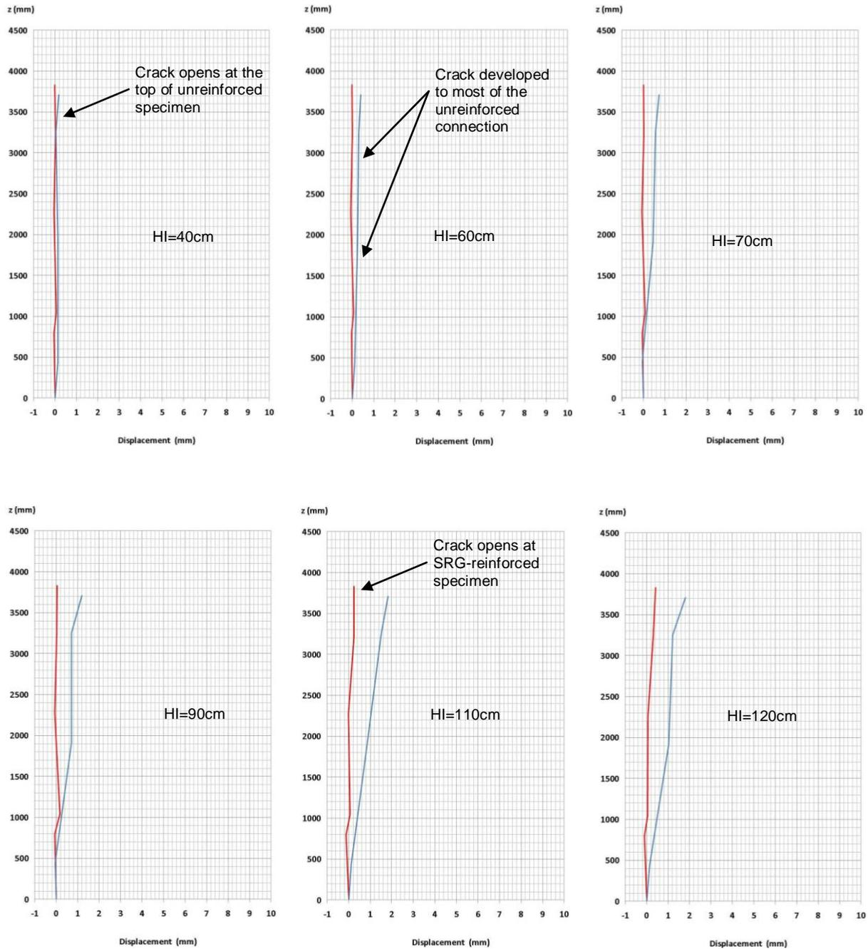
Figure 9: Evolution of south wall-façade connection after shaking table tests at different HI values: Red profiles correspond to SRG-reinforced specimen
