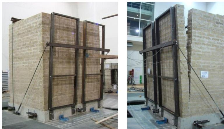
Figure 2: Unreinforced specimen: before shaking table tests (left) and out-of-plane collapse of the façade (right).
