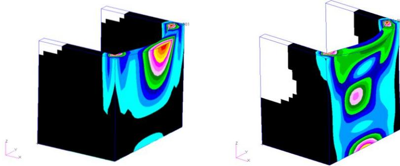
Figure 5: FE Model (left), first modal shape (center), second modal shape (right).
