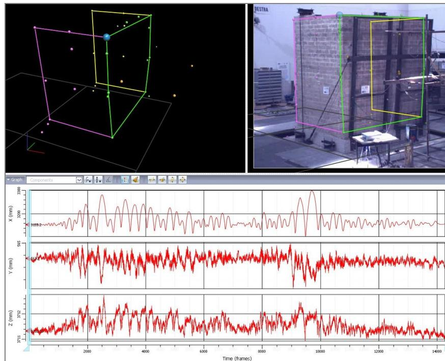
Figure 7: Real-time monitoring of a 3DVision marker: x, y and z trajectory components (bottom graphs) of the selected marker (enhanced in blue in top left and right).
