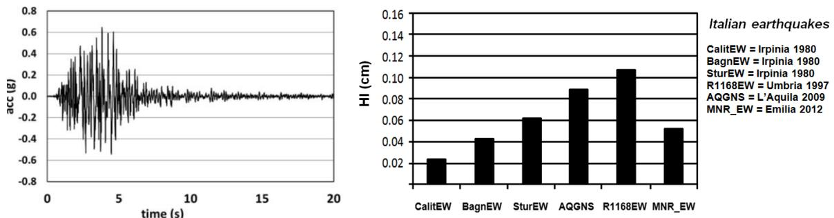
Figure 8: Input R1168EW based on Umbria–Marche earthquake of September 1997 (left), and comparison of the main Italian earthquakes since 1980 in terms of HI computed in the range 8-16 Hz (right).
