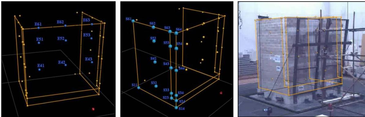
Figure 6: Positions of 3DVision markers: façade (left), south wall (center) and 3D Overlay (right).
