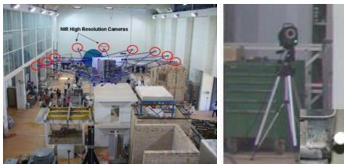
Figure 1: 3DVision system: typical configuration of NIR cameras in the lab (left); detail of a NIR camera (right).
