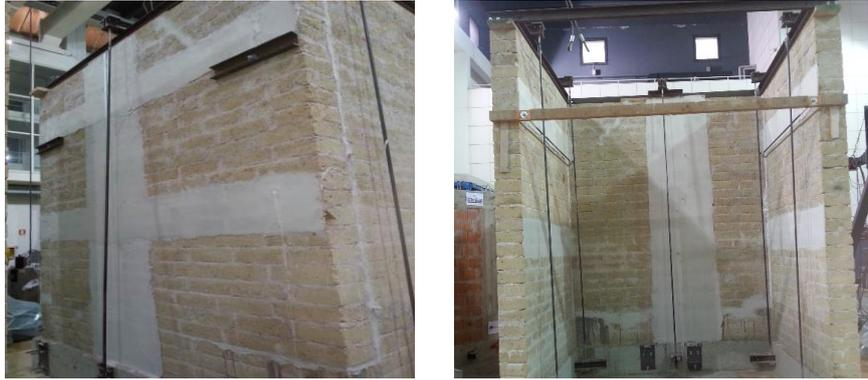
Figure 3: SRG-reinforced specimen: façade (left) and back view (right).
