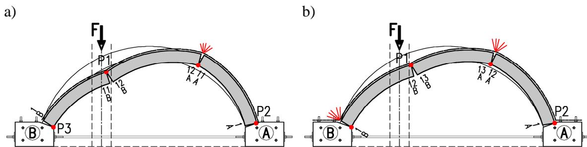
Figure 6: Failure mechanisms observed during the tests: a) vault VG2, b) vault VG-An.
