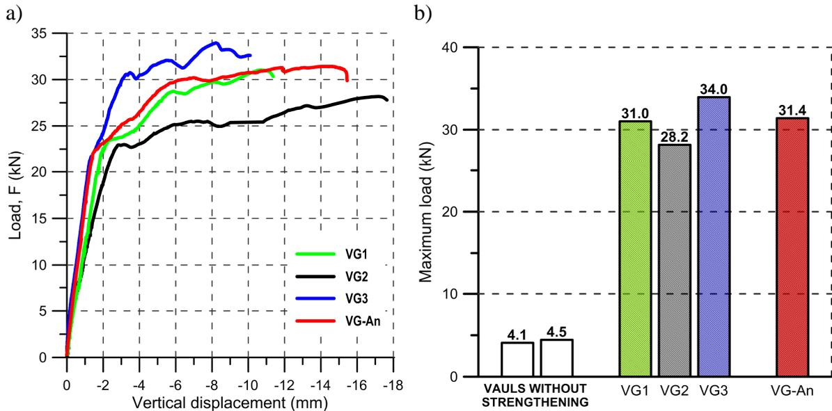
Figure 5: a) Load – vertical displacement (at the point of loading) curves for the tested vaults. b) Maximum loads for the tested vaults – summary.
