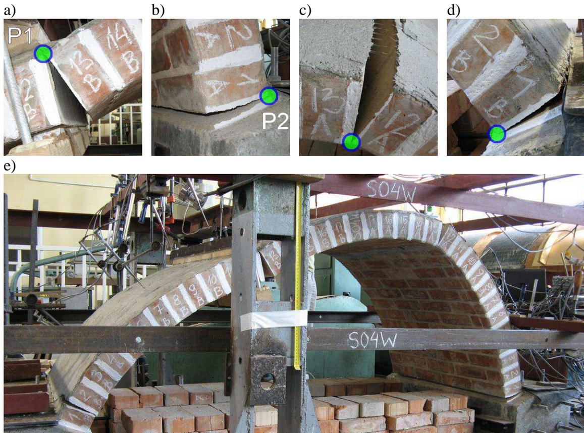
Figure 4: Vault VG-An (originally named S04W): a)-d) cracks and hinges of the collapse mode, e) failure mechanism.
