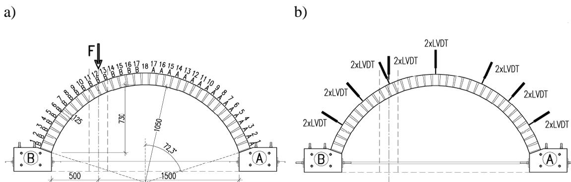
Figure 1: a) Geometry of the tested vaults, brick course numbering. b) Instrumentation arrangement, (dimensions in mm; LVDT – displacement transducers).
