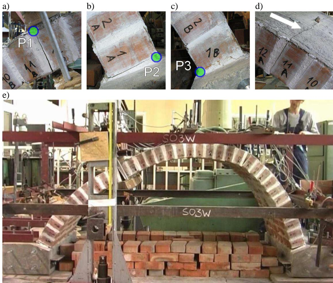
Figure 3: Vault VG2 (originally named S03W): a)-c) cracks and hinges developed, d) crack at the extrados – ruptured glass fibers, e) failure mechanism.
