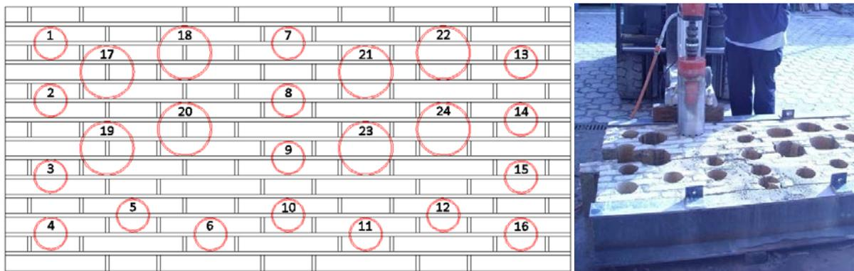
Figure 3: (a) Location of cylinders in the wall, (b) extraction of specimens.
