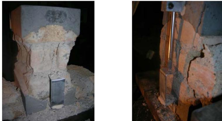
Figure 10: Typical regular failure at the end of the test (a) and failure with crack involving the cap (b).
