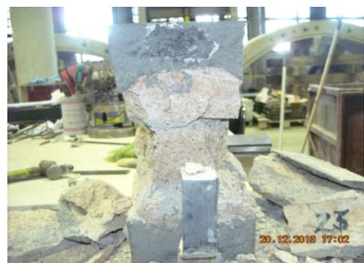
Figure 9: Stress-strain curves of two joint specimens (a) and mode of failure (b).
