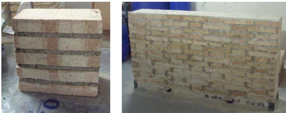
Figure 2: (a) Stack prism and (b) wall used for core drilling.
