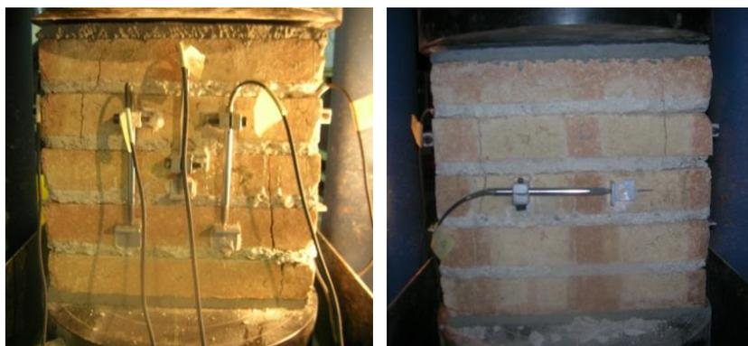
Figure 7: Damage in stack prisms after testing.
