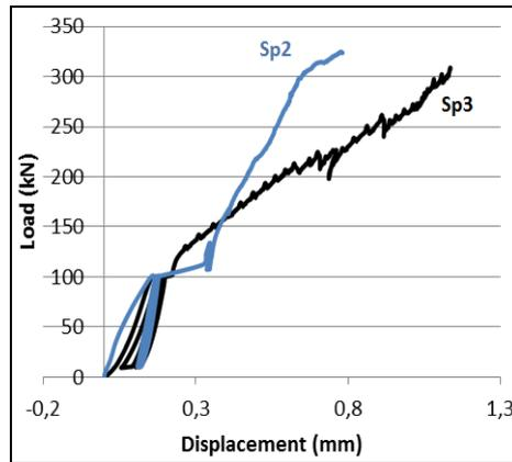
Figure 6: Load-Displacement curves of stack prisms 2 and 3
