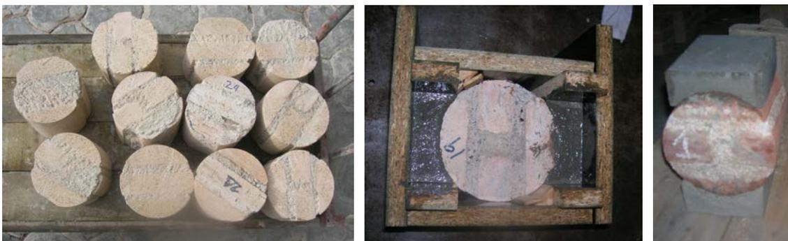
Figure 4: (a) Three and two joint cylindrical masonry samples, (b) mould used for the regularization of the specimens, (c) regularized specimen ready to be tested.
