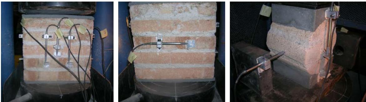
Figure 5: (a, b) Stack prisms and (c) regularized cylindrical specimen before the test.
