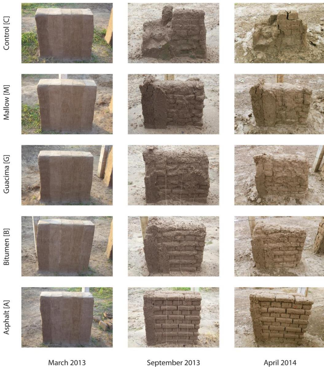
Figure 4: Monitoring of Phase 1 test walls (Photos: Kita).
