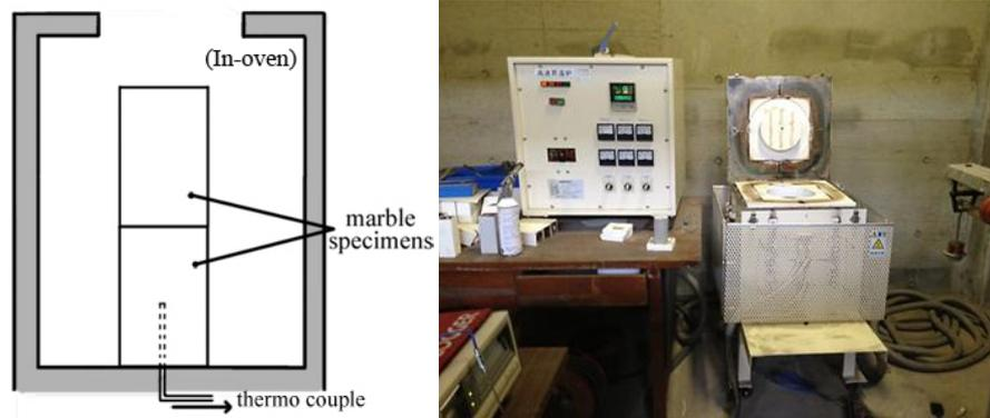
Figure 1: Electric furnace and specimen
