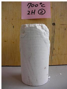
Figure 7: Deterioration of specimen with time. (After 60 hours from the end of heating at 700°C for two hours)
