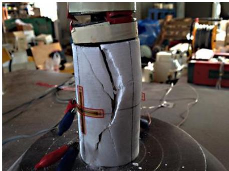
Figure 10: Failure mode (un-heated specimen)
