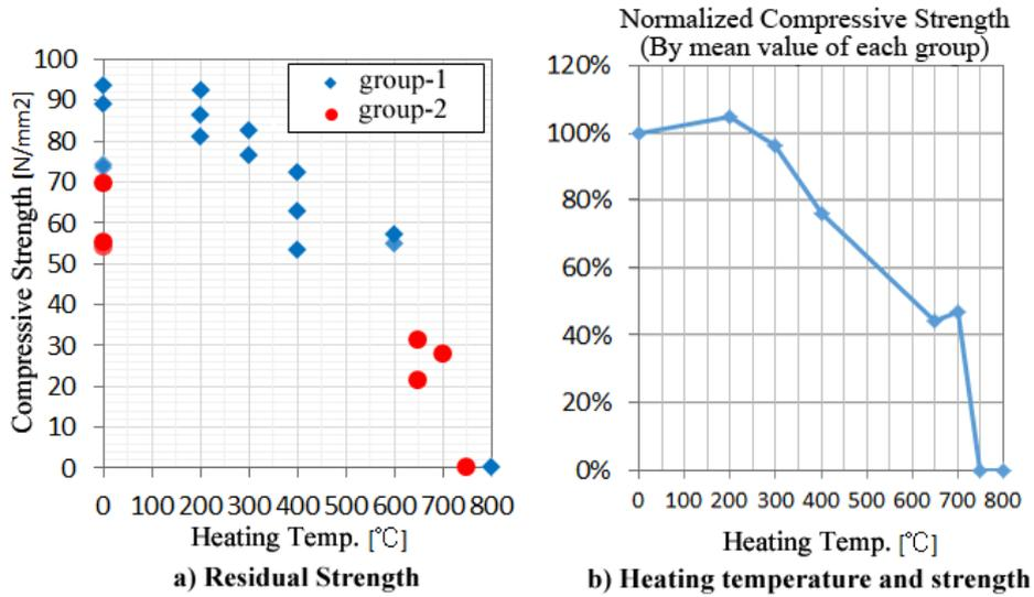
Figure 9: Relation between heating temperature and strength
