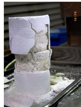
Figure 8: Surface layer of specimen exfoliated. (After 120 hours from the end of heating at 800°C for two hours)
