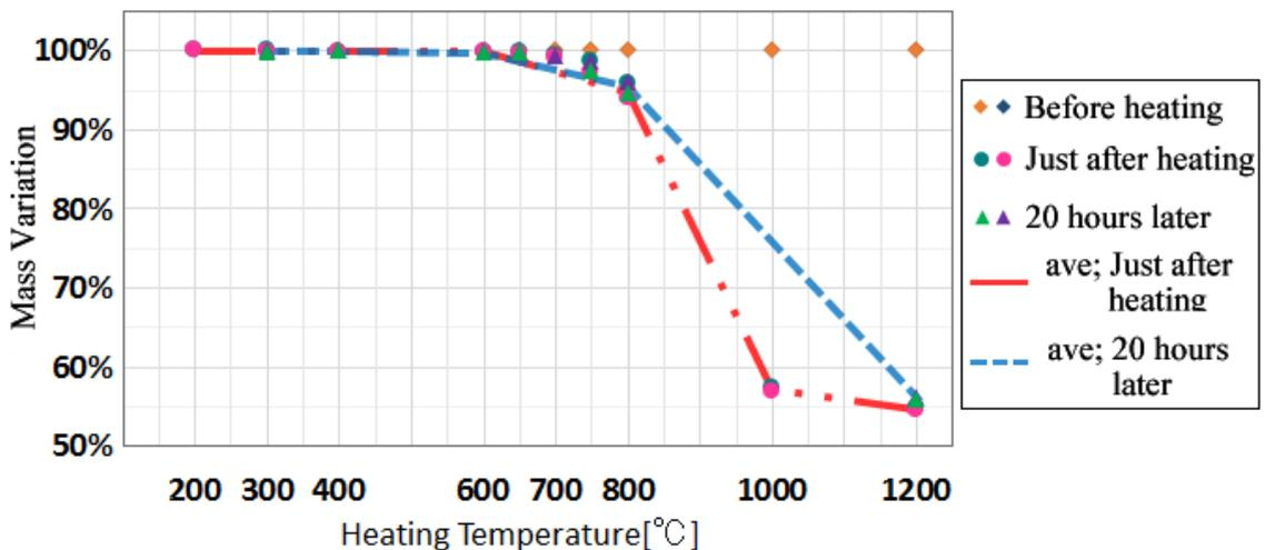
Figure 5: Relation heating temperature and mass variation with Constant Temperature Tests.
