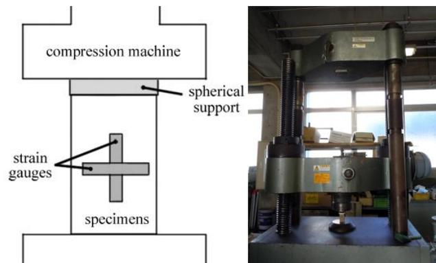
Figure 2: Compression test
