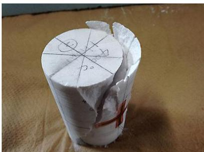
Figure 12: Detail of failure mode (heated specimen at 400°C)
