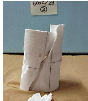
Figure 11: Failure mode (heated specimen at 600°C)
