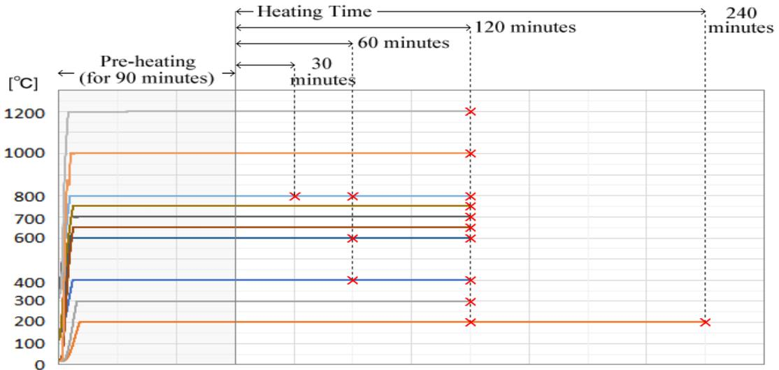
Figure 3: Controlled Temperature of heating tests
