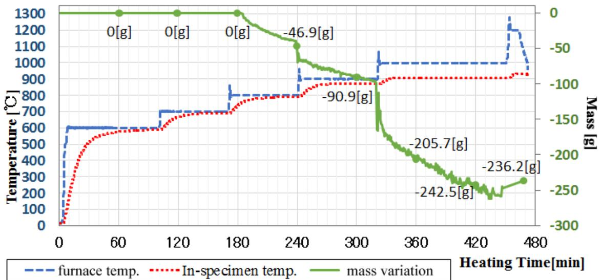
Figure 4: Mass variation with time in step heating test by raising 100°C.
