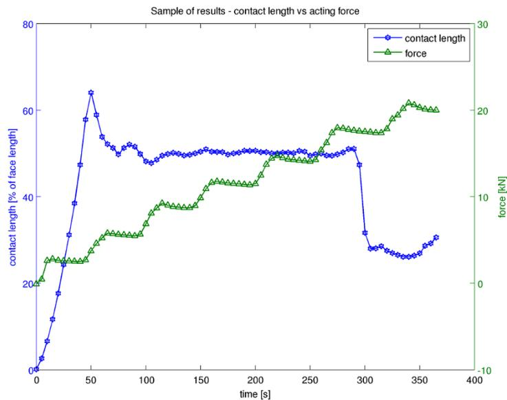
Figure 3. Contact length and acting load in time.
