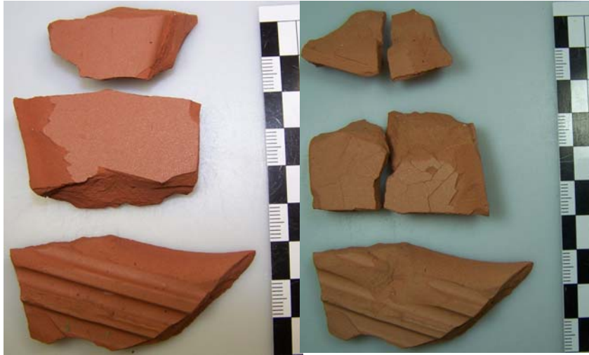
Figure 6. Brick specimens B1-B3 before (left) and after (right) 25 cycles of freezing/thawing tests.
