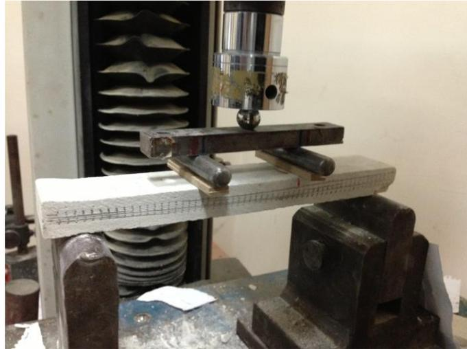
Figure 3: Flexural loading test setup.
