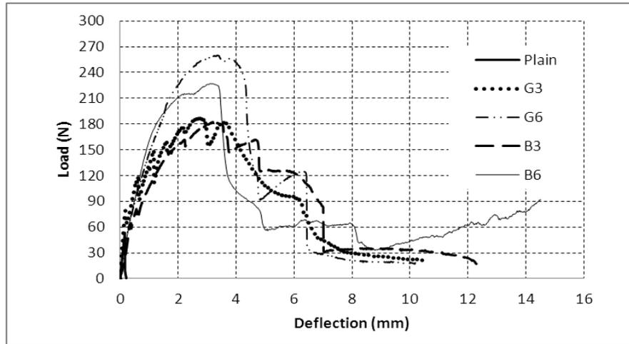
Figure 6: Typical behavior of textile reinforced lime composites under flexural loads.
