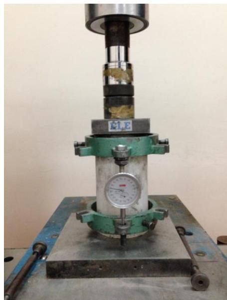
Figure 4: Test setup for compressive tests.
