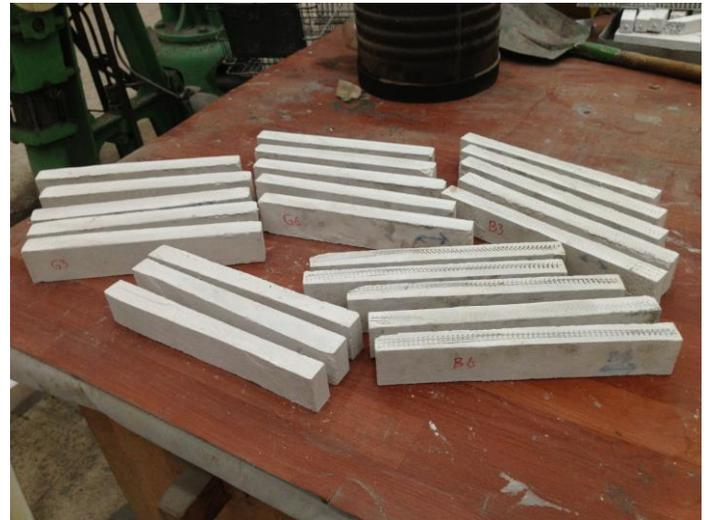
Figure 2: Specimens prepared for flexural tests.
