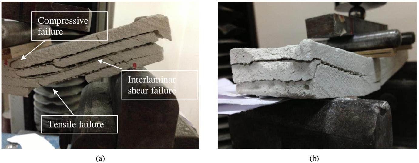
Figure 8: (a) Multiple cracks occurred in the specimens (b) Laminated failure of the specimens.
