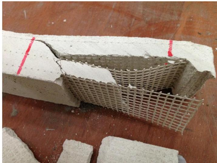
Figure 9: A glass textile reinforced lime composite specimen after test.
