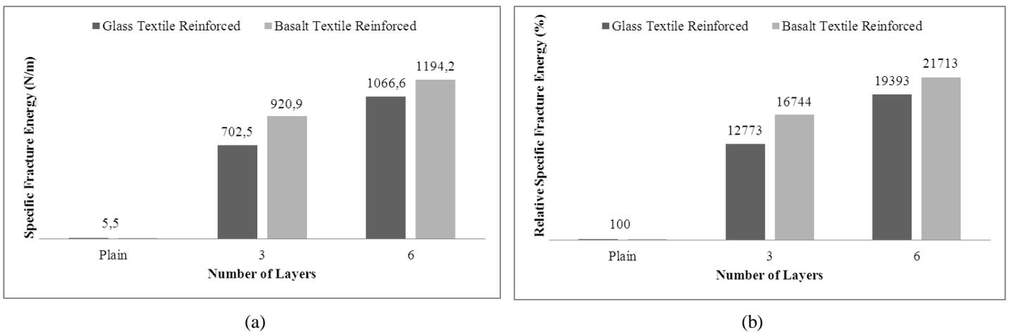
Figure 7: Variation of the specific fracture energy of the composites by reinforcement type and amount.
