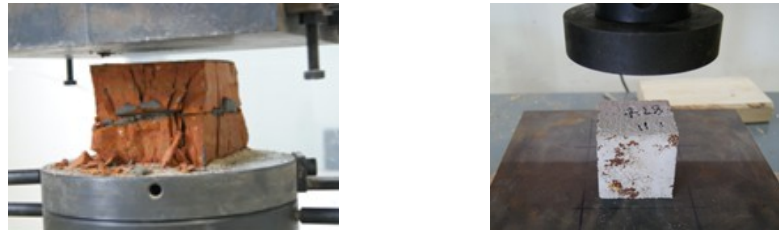
(a) Compression test of brick specimens (b)Compression test of mortar specimens
