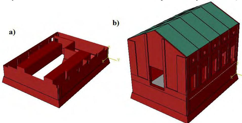
Figure 3: Numerical modeling of the chapel: a) foundation blocks, b) the whole 3D model.
