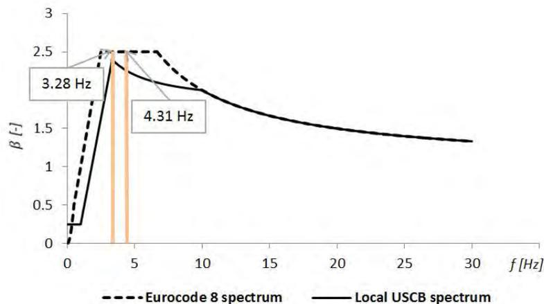
Figure 7: The shapes of the horizontal response spectrum recommended in EUROCODE 8 and the local spectrum established for the USCBA region with two lowest natural frequencies.
