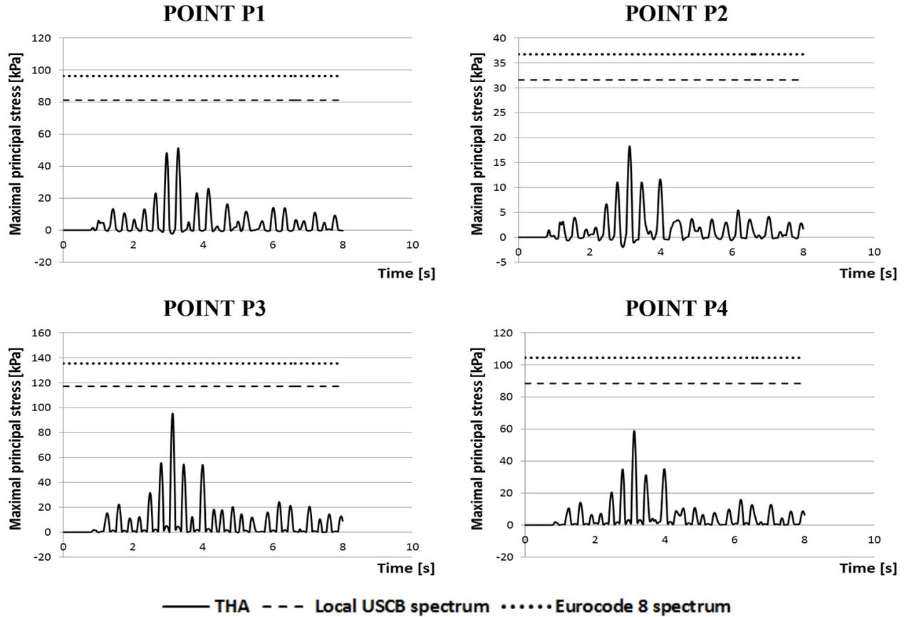
Figure 11: Relation between maximal principal stresses at points P1-P4 (see Fig. 9) obtained from *THA* and *RSA* method with the EUROCODE 8 elastic spectrum and the local LGCD elastic spectrum.
