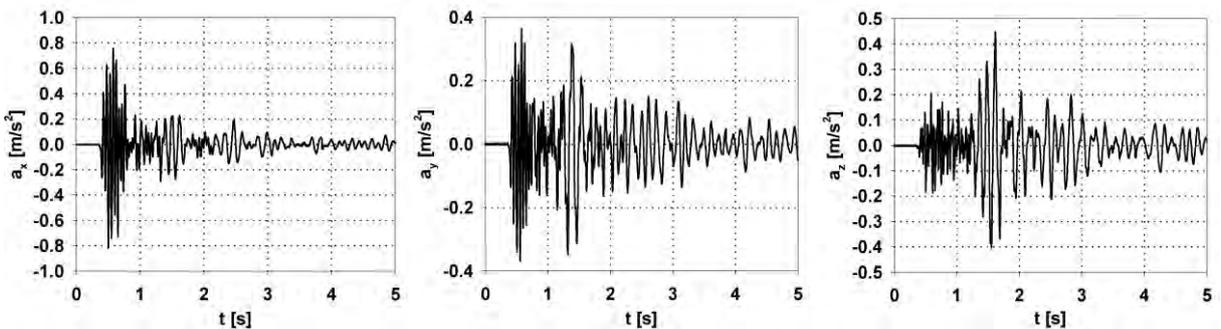
Figure 5: Time histories of ground motion accelerations registered in the LGCD region in three directions:  $a_x, a_y$  – horizontal, orthogonal;  $a_z$  – vertical.
