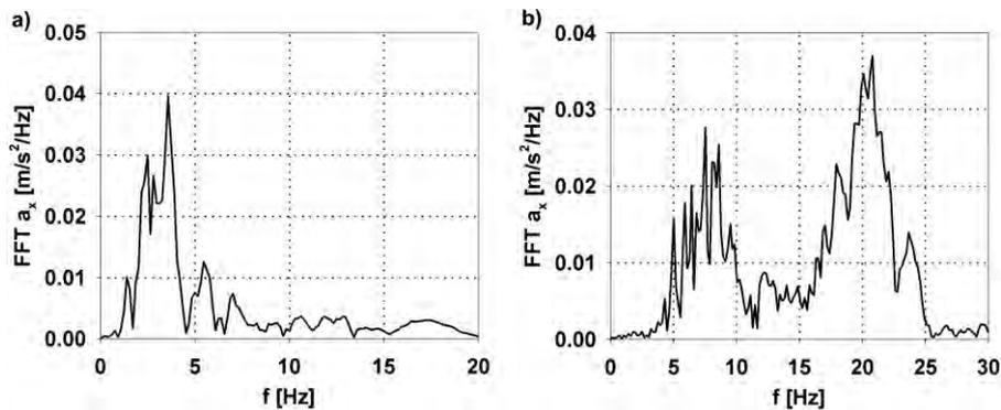
Figure 6: The frequency spectra of the mining shock registered in horizontal direction X in: a) the USCBA region, b) the LGCD region.
