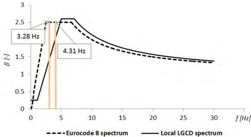
Figure 8: The shapes of the horizontal response spectrum recommended in EUROCODE 8 and the local spectrum established for the LGCD region with two lowest natural frequencies.
