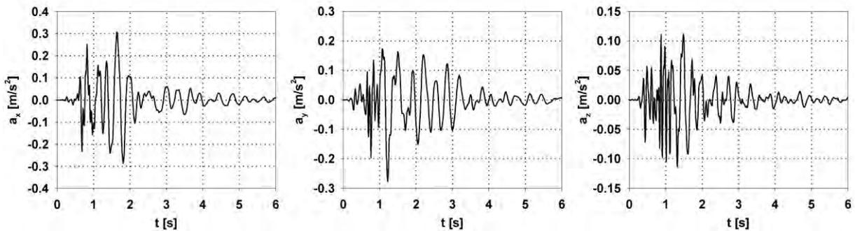
Figure 4: Time histories of ground motion accelerations registered in the USCB region in three directions:  $a_x, a_y$  – horizontal, orthogonal;  $a_z$  – vertical.
