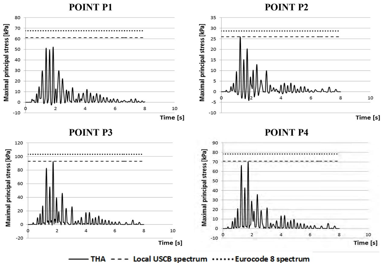
Figure 10: Relation between maximal principal stresses at points P1-P4 (see Fig. 9) obtained from *THA* and *RSA* method with the EUROCODE 8 elastic spectrum and the local USCB elastic spectrum.
