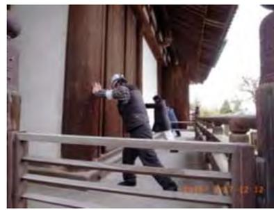
Photo.5 Free-Vibration test by man-power
