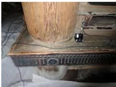
Photo.4 Sensors on the base beam
