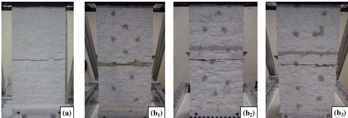
Figure 3: Typical failure modes observed: (a) before grouting, and after grouting for (b<sub>1</sub>) specimen founded on a rigid base, (b<sub>2</sub>) specimen founded on dense sand, and (b<sub>3</sub>) specimen founded on loose sand.
