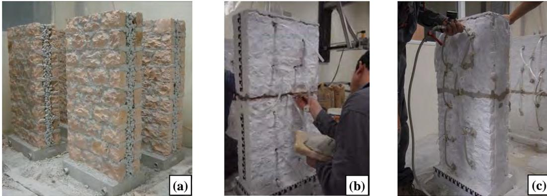
Figure 1: Wall-footing specimens: (a) as-built, (b) during the application of deep repointing, and (c) during the application of grout injections.
