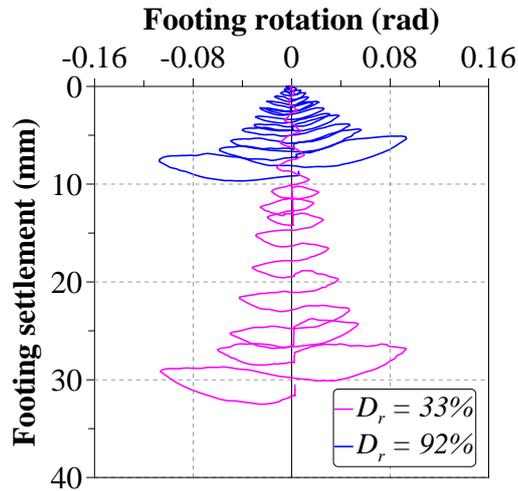
Figure 2: Footing settlement–rotation response: comparison between dense sand ( $D_r=92\%$ ) and loose sand ( $D_r=33\%$ ).
