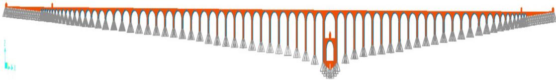
Figure 16: Finite element model of the whole bridge.
