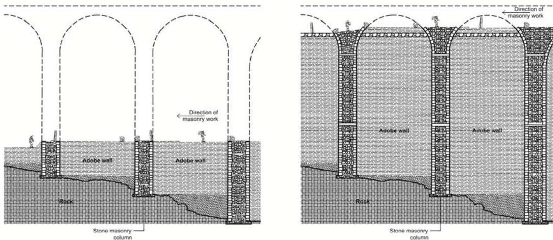
Figure 5: Building procedure for the highest segment of the arched bridge.
