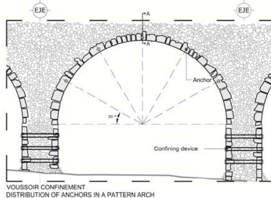
Figure 23: Location of confining devices for columns and arches.
