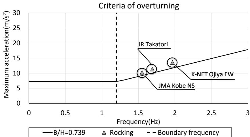
Figure 13: Rollover limit acceleration and movement pattern in input seismic wave.
