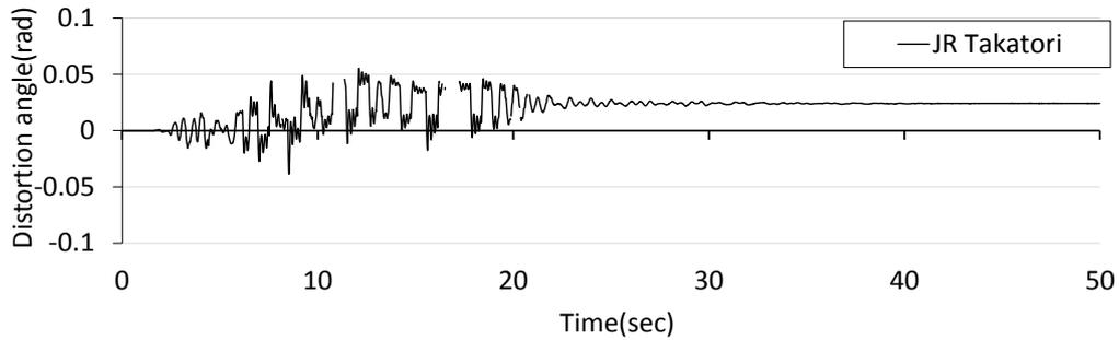
Figure 11: Waveform of deformation angle time history.
