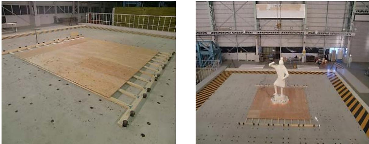
Figure 7: Floor installed on the vibrating table.
