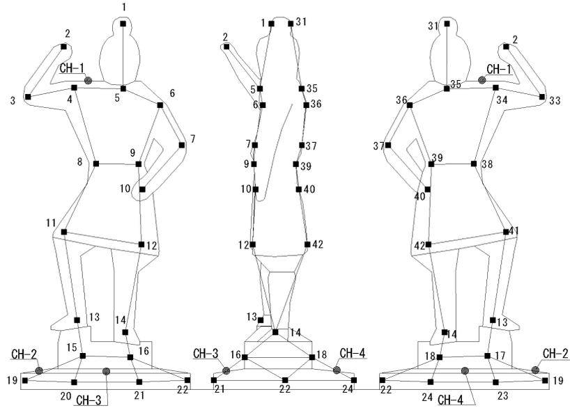
Figure 8: Accelerometer and light-emitting marker installation positions.
