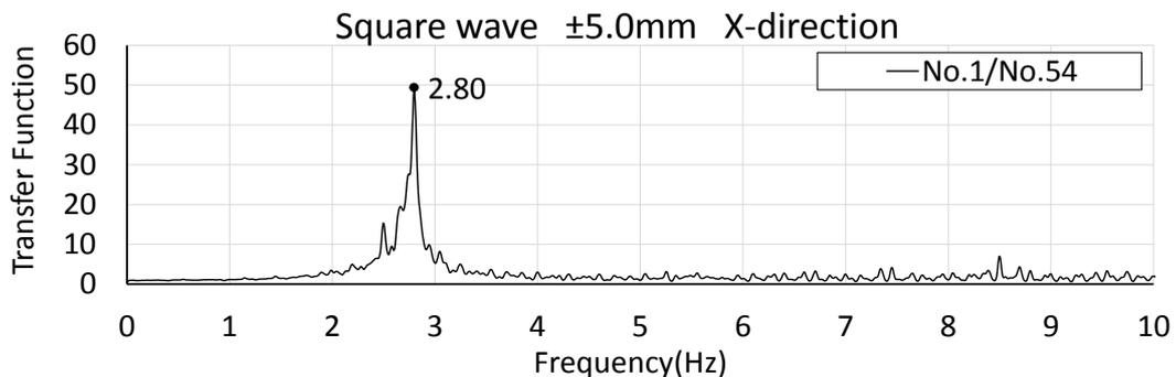
Figure 9: Transfer function of the head with respect to the vibrating table.
