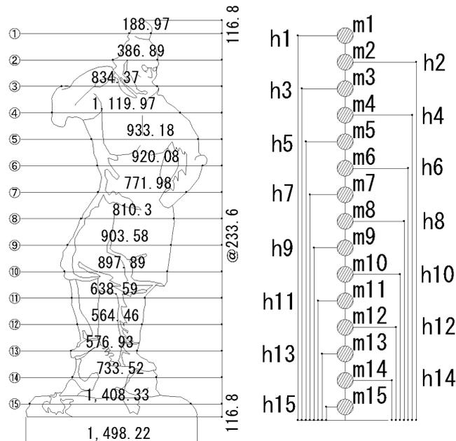
Figure 5: Split locations used for center gravity height calculation.
