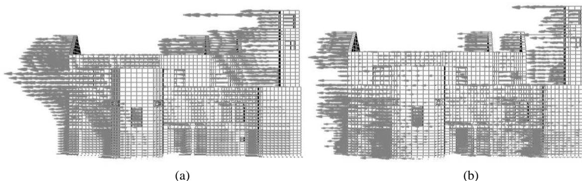
Figure 4: Load in positive X direction (a) Nodal load distribution for load case G1 (b) Nodal load distribution for load case G2.
