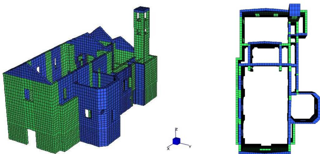
Figure 3: 3-D model of Rosario Church (Nodes= 19275 Elements=9076).
