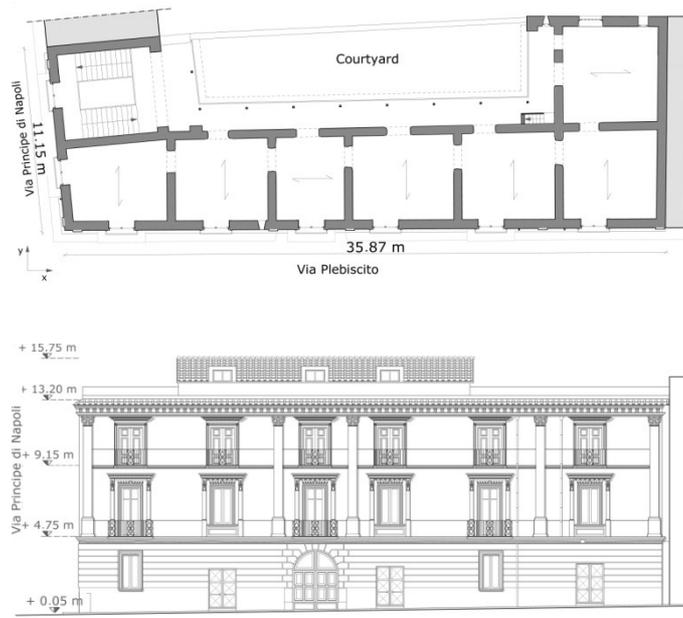
Figure 2: Plan and elevation layouts of Pelella Palace.
