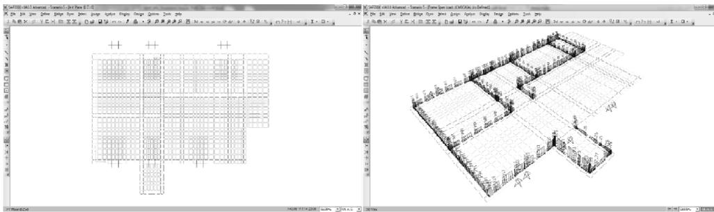
Figure 5 Bar element model of waffle slab and uniform distributed loads [7]
