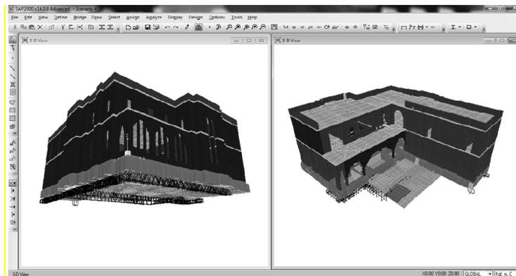
Figure 6 Finite element model of the historical house [7]
