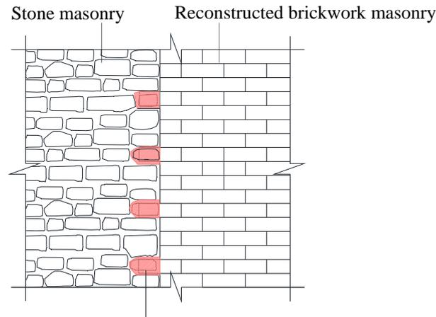
Removal of stones (locally) and achievement of interlocking between stone masonry and brickwork masonry
