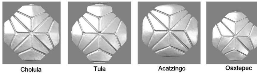
Figure 3: Horizontal section of the vaults at the height of the keystone of the perimeter ribs.
