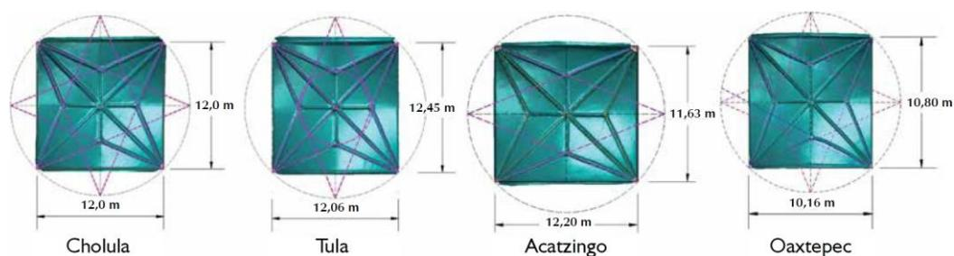
Figure 4: Trace of tiercerons in plan.
