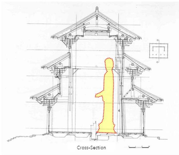
*fig 1 Section drawing of the Mireukjeon Hall of Gumsansa Temple, Gimje*
