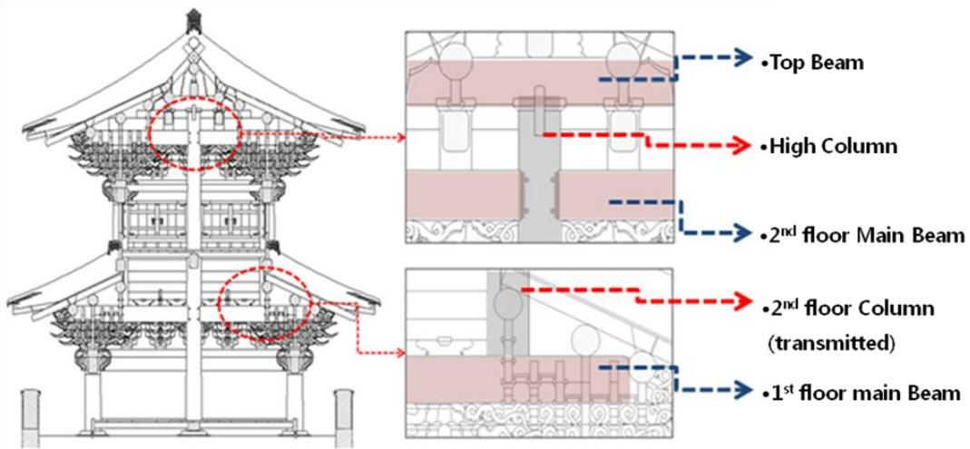
fig 4 Section of Hunginjimun Gate and structural system of main element
