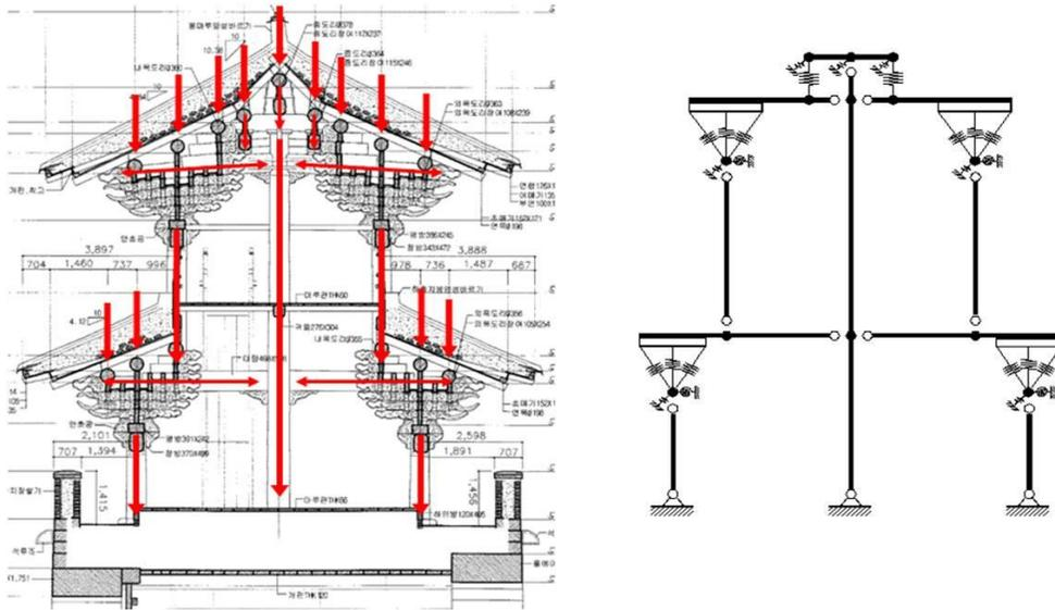
fig 5 Axial force diagram and simplified model of section
