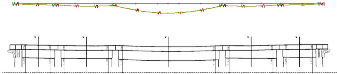
fig 9 Deflection of 3D model (top) and actual survey (bottom)
