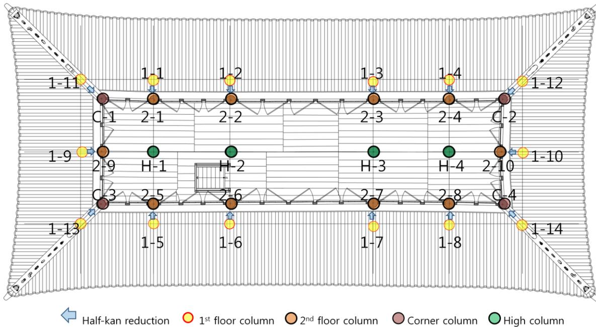
fig 3 2nd floor Plan and column arrangement of Hunginjimun Gate
